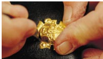
9 CHASING then applied details to the front of the object.
