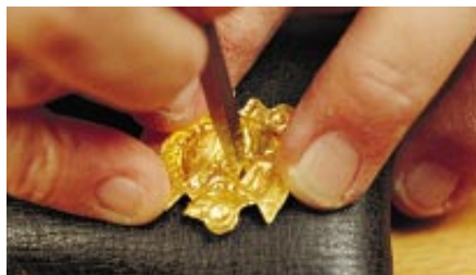
8 REPOUSSÉ, employing another tumbaga tool, pushed up the gross form. The piece was worked against the resistant surface of a leather sandbag.
